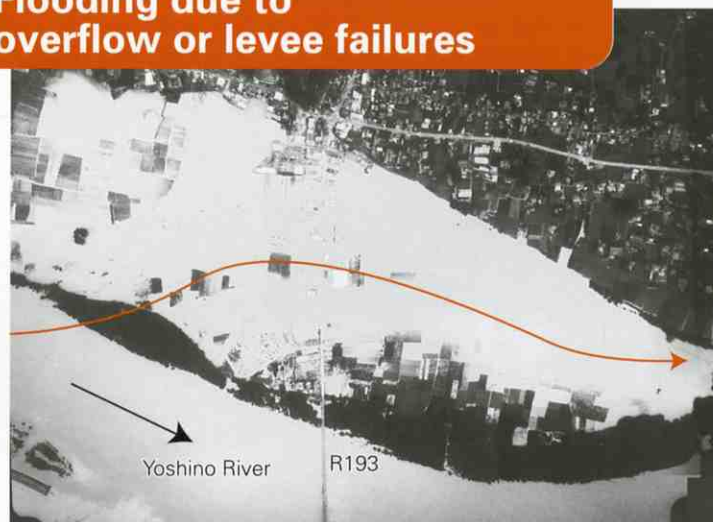
The flood of 1974 caused serious damage because there were no embankments along Waki Town.
