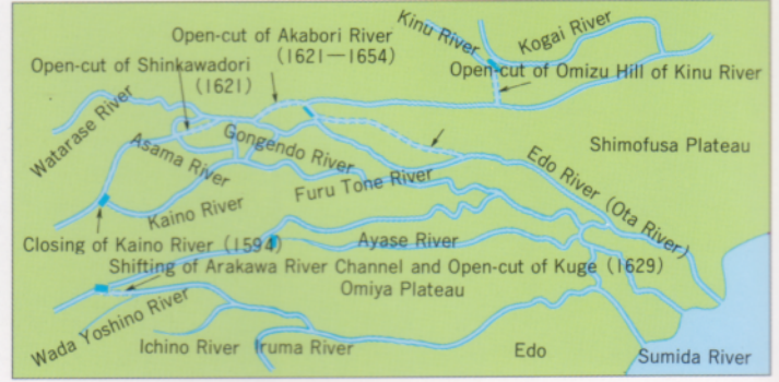
Eastward shift of Tone River and excavation of Edo River
