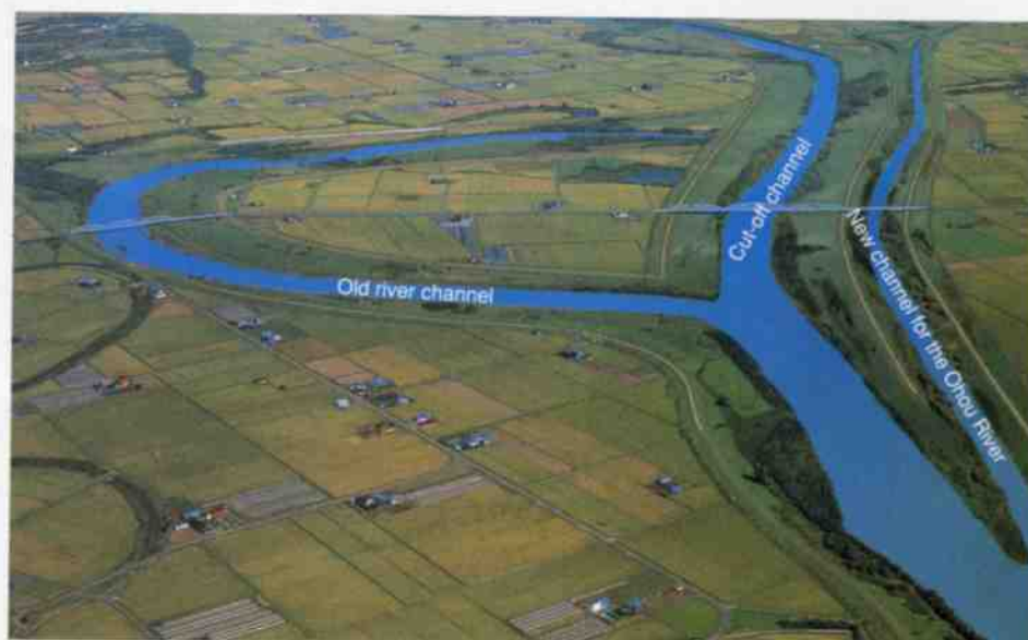
Projected image when the cut-off channel is completed
