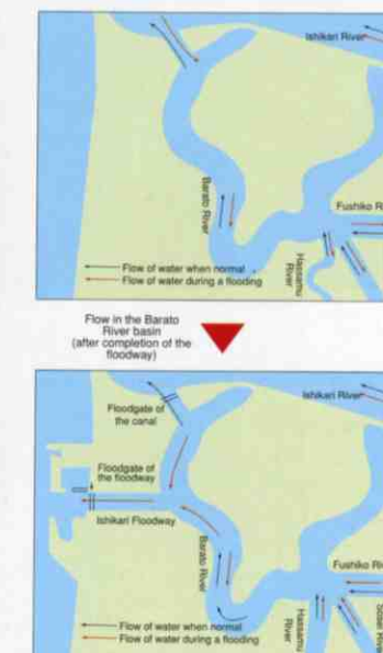
Figure 35 Schematic diagram of the floodway
