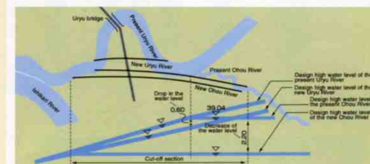
Figure 26 Decrease of the water level with the cut-off channel (cut-off channel of the Uryu River)
